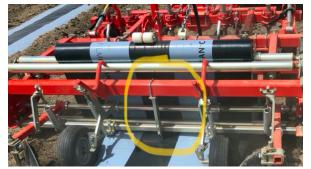
Make sure the vertical bar does not score or tear the mulch film.
